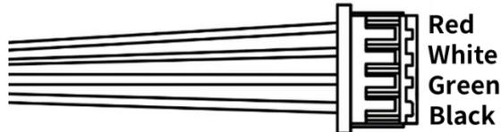
Figure 2-1 TF02-Pro external wiring connector and wiring sequence
