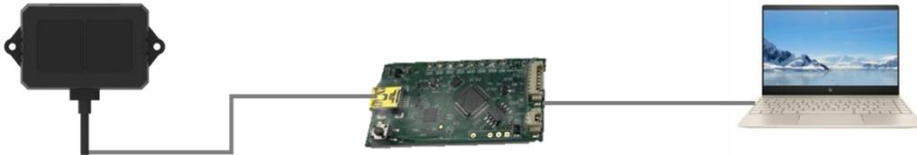
Figure 5-1 Connection of TF02-Pro and PC
